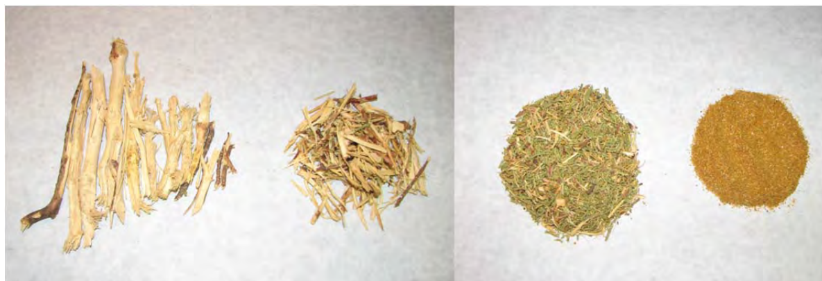
Fig. 7. Particle distribution of a supplement (control) separated by the Penn State Particle Separator; left to right: material remaining on 19.0, 8.0, and 1.18-mm sieves, and in bottom pan (< 1.18 mm).
