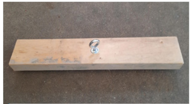
Figure 4. Example of a standard threaded eye-bolt with flat washers on both sides. Photo courtesy of Costanzo, Texas A&M AgriLife, 2021
