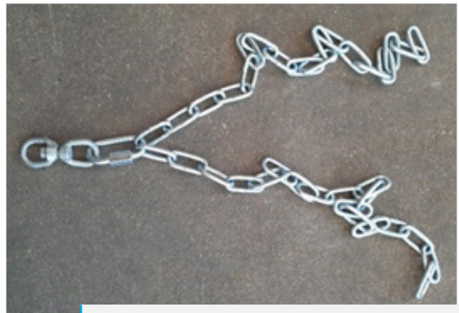
Figure 13. Quick link and swivel attached to chains.
