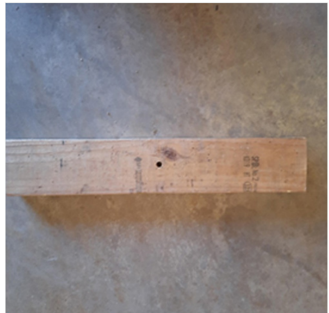
Figure 3. The location to drill a hole for the eye-bolt, which is slightly larger than the diameter of it. Photo courtesy of Costanzo, Texas A&M AgriLife, 2021
