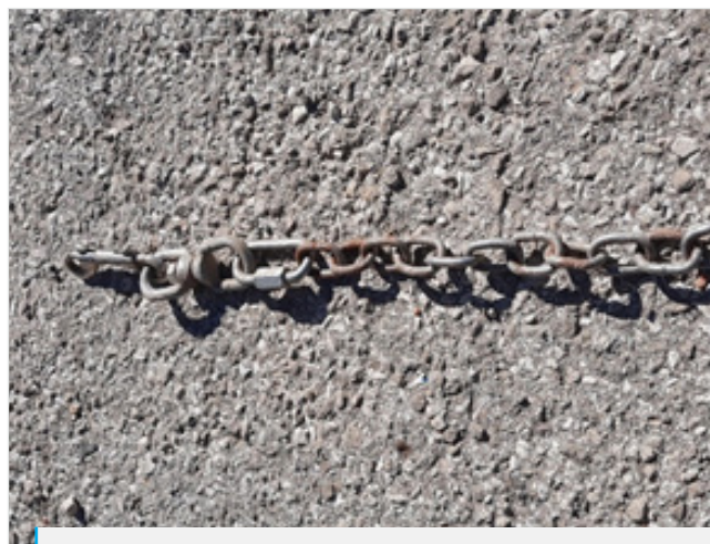
Figure 11. A chain with two quick links and swivel attached. Photo courtesy of Costanzo, Texas A&M AgriLife, 2021
