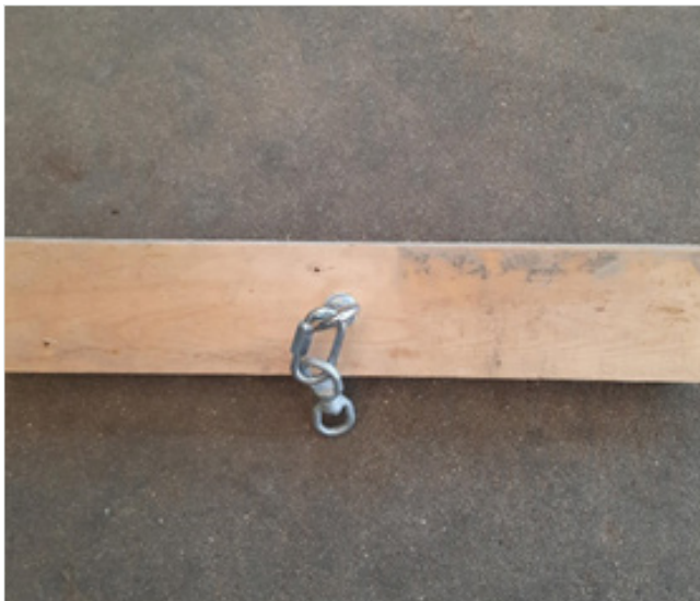
Figure 5. An attached quick link and swivel tightened to the eye-bolt loop. Photo courtesy of Costanzo, Texas A&M AgriLife, 2021
