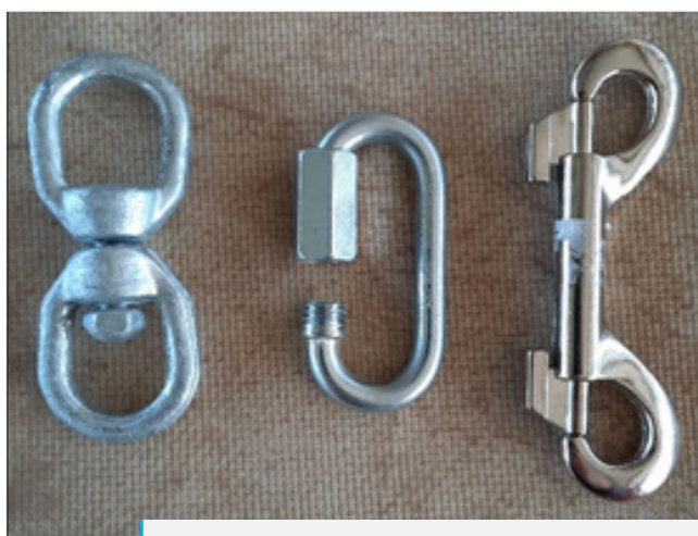
Figure 9. Swivel, quick link, and double-end snap. Photo courtesy of Costanzo, Texas A&M AgriLife, 2021
