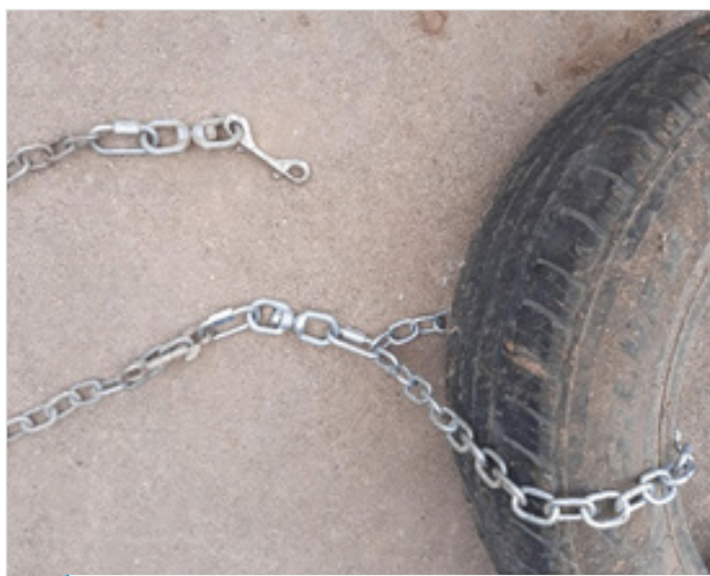
Figure 8. Tire drag with swivels at each end of the chain. Photo courtesy of Costanzo, Texas A&M AgriLife, 2021
