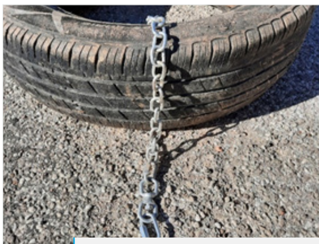
Figure 10. A tire drag with quick link and swivel. Photo courtesy of Costanzo, Texas A&M AgriLife, 2021
