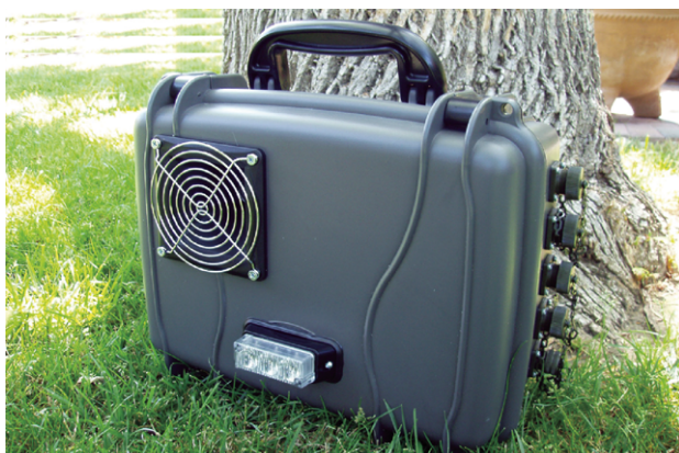
Figure 3. The ScareCall, a fully programmable light and sound device that can be suspended on a fence or tree in a pasture to prevent the advance and intrusion of wary carnivores. The device can use randomly activating lights and repellent sound effects (e.g., gunfire), or can be programmed with attractant calls (e.g., prey distress calls) to draw predators into an area for capture. Photograph: Martin Lilly, ML Designs.
