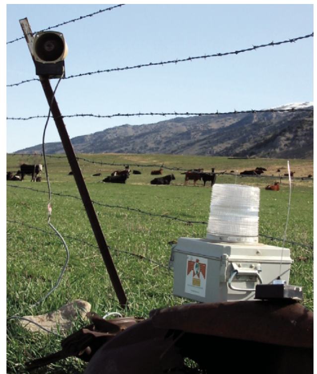
Figure 4. The radio-activated guard (Avian Systems Model 9000 frightening device). When a radio-collared predator approaches the area, the strobe light activates, along with a series of 30 sound effects. Photograph: John Shivik, US Department of Agriculture.
